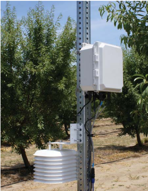
PureSense field stations measure above- and below-ground conditions every 15 minutes. Data is transmitted to a secure server and compiled into easy-to-use, customized charts and reports to help growers plan, schedule and precisely manage their irrigation activities.
